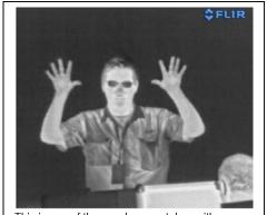
This image of the speaker was taken with an uncooled microbolometer camera operating the 7-14 micron waveband
