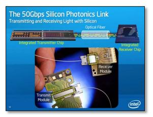
Photonics has transformed our experience with the Internet through low-cost, high-bandwidth fiber optic transmission. The next level of evolution, integrated optics or "silicon photonics" combines electrical and optical components on the same silicon-based substrates that are used in the fabrication of a semiconductor chip. Lasers, photodetectors, beam splitters, isolators, filters, prisms, modulators and optical switches can be designed into the same microchip.
