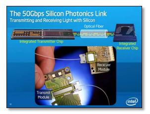
Photonics has transformed our experience with the Internet through low-cost, high-bandwidth fiber optic transmission. The next level of evolution, integrated optics or "silicon photonics" combines electrical and optical components on the same silicon-based substrates that are used in the fabrication of a semiconductor chip. Lasers, photodetectors, beam splitters, isolators, filters, prisms, modulators and optical switches can be designed into the same microchip.
