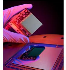
covering the x-ray, visible, infrared, terahertz, and millimeter wave regions of the electromagnetic spectrum. This presentation will provide a basic understanding of the ReadOut Integrated Circuits (ROIC) designed for infrared and visible focal plane array (FPA) sensors. Key imaging characteristics will be introduced, like spectral content, type of detector covering specific wavelength bands (HgCdTe and Si) and basic ROIC front-end architectures.
