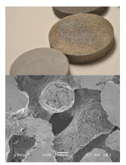
The Shape Memory Effect (SME) in certain metals are due to phase transformations that occur when the material is heated or cooled through a set of transformation temperatures. One SME alloy in particular, Nitinol, has seen as great deal of interest as these transformation temperatures can be modified easily by small changes to the Ti:Ni ratio and by the introduction of dopants, making them suitable for both industrial and biomedical applications.
